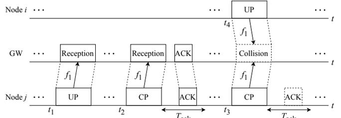
Fig. 1. Time-sequence example in conventional LoRaWAN
