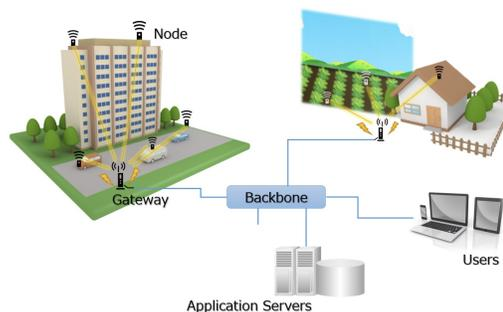
Fig. 1. In LoRaWAN architecture, nodes communicate to the network server through gateways.
