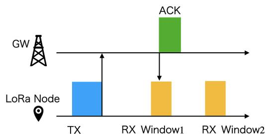
Fig. 2. LoRaWAN protocol on Class A.
