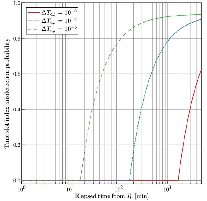
Fig. 3. Impact of clock drift on misdetection probability of time slot index.
