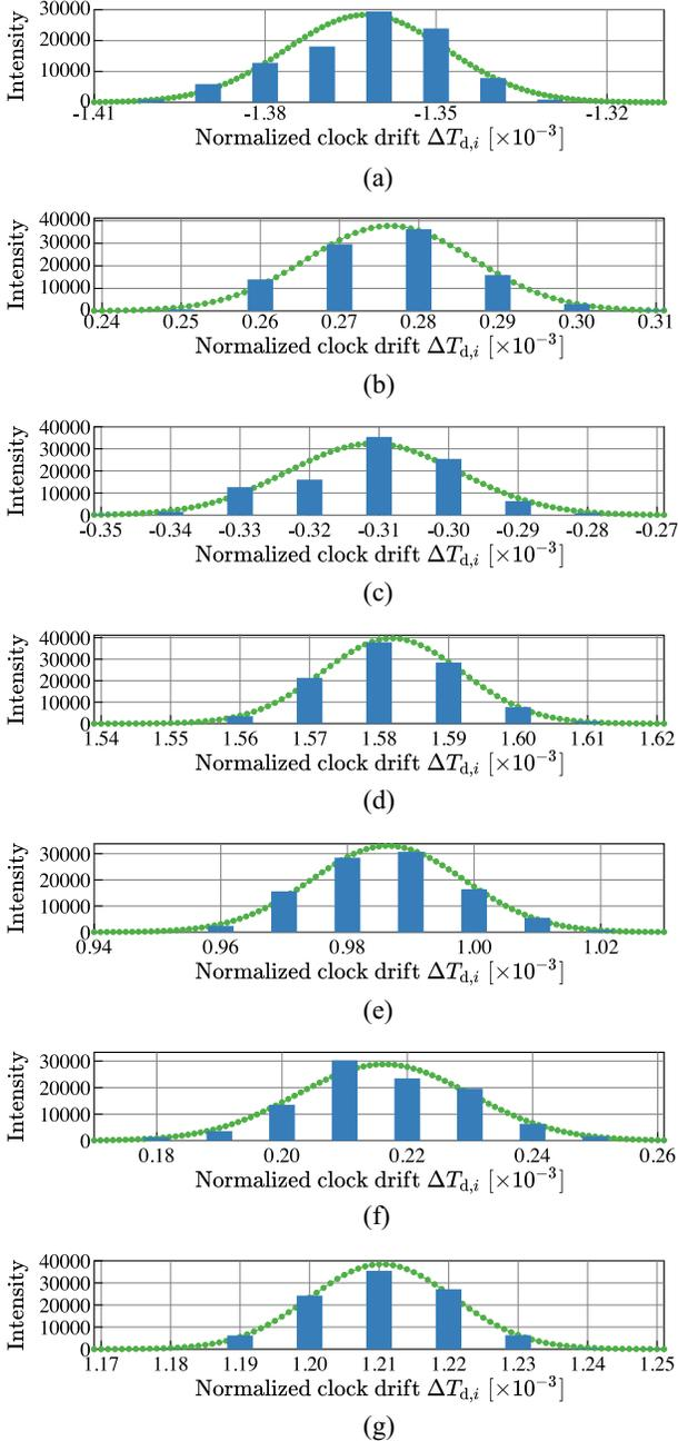
Fig. 4. Measurement results of relative clock drift between Dragino LG-01 and LoRa Mini Dev-JP. (a) EN 1. (b) EN 2. (c) EN 3. (d) EN 4. (e) EN 5. (f) EN 6. (g) EN 7.
