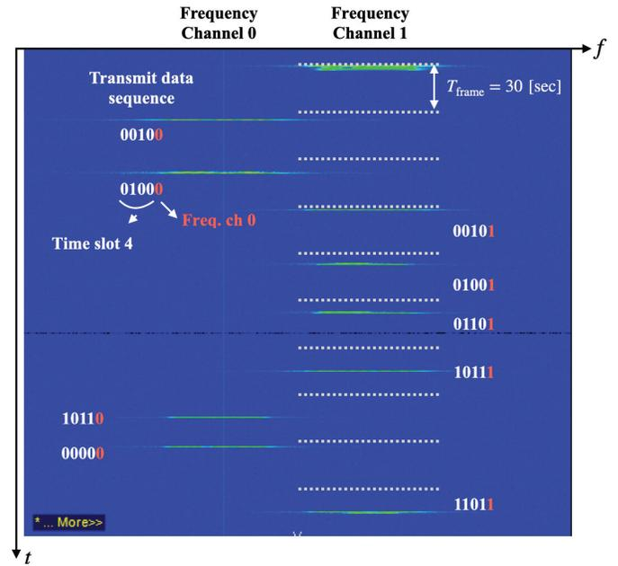
Fig. 8. Spectrogram of LoRaWAN with PLIM.
