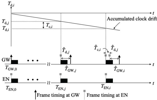
Fig. 7. Example of clock drift compensation with  $\mu < 0$  and  $\sigma^2 = 0$ . As an example, we set  $q_j = q_i = 0$ .
