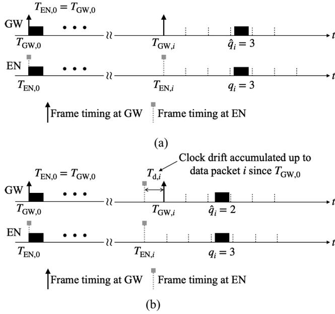
Fig. 2. Index misdetection due to clock drift when  $T_{d,i} < 0$ . (a) Without clock drift. (b) With clock drift.
