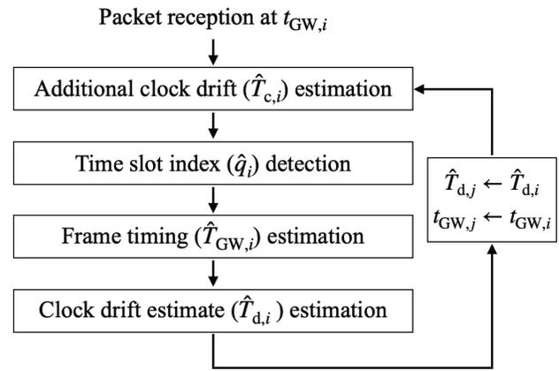
Fig. 6. Flowchart of clock drift estimation and compensation at GW.
