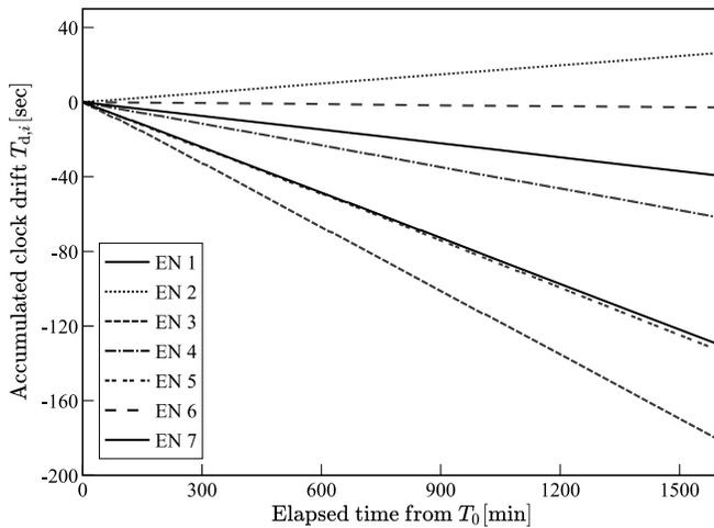
Fig. 5. Accumulated clock drift of seven ENs as a function of the elapsed time from  $T_0$ .
