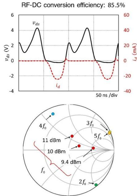
Fig 2.4-6 Example of the active source-pull for a GaAs HEMT at 10 MHz. Upper Fig.: vottage and current waveforms, and lower Fig.: estimated source impedances
