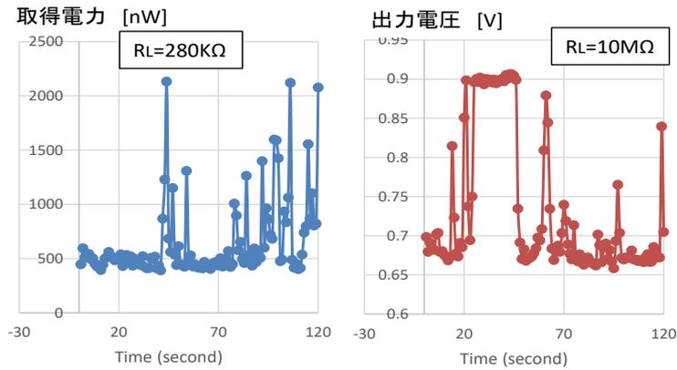
Figure 2.4-3 Output power and voltage from environmental RF energy of 950MHz for cell phones.
