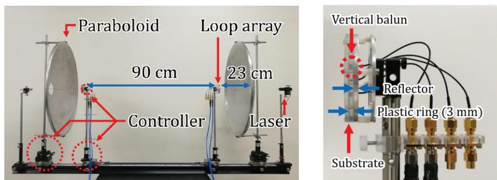
Fig. 2.2-13 Long-range OAM communication system using loop antenna arrays at 12-GHz band.
