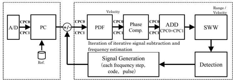
Fig.2.1-10 Block diagram of the signal processing of iterative signal subtraction and frequency estimation method in stepped multiple frequency CPC.
