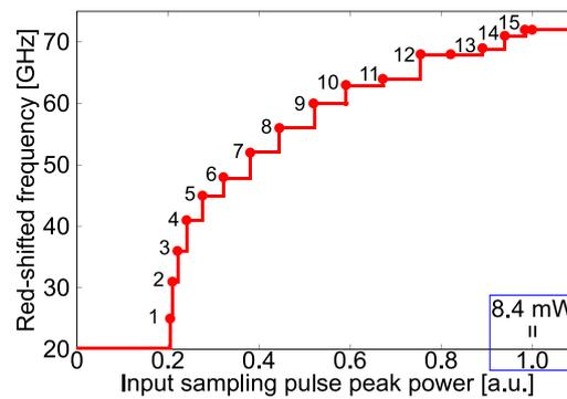
Fig.2.2.14 15-level quantization performance
