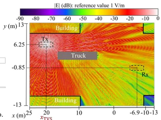
Fig. 2.1-7 Electric field strength map in intersection.
