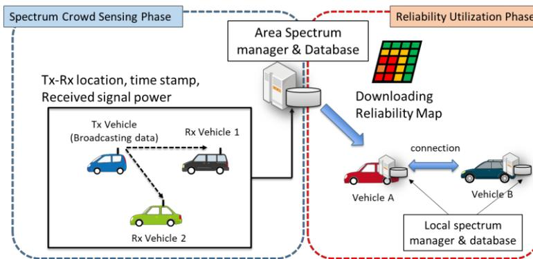
Figure 2.1-1 Concept of spectrum database with communication reliability.
