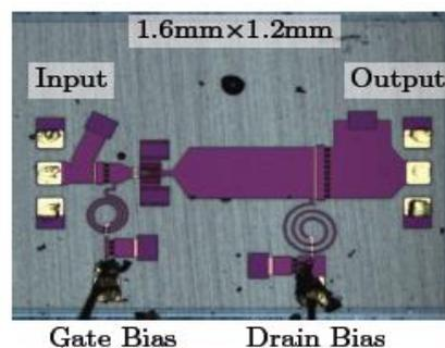
Fig 2.2-2 28GHz-band GaN HEMT MMIC power amplifier
