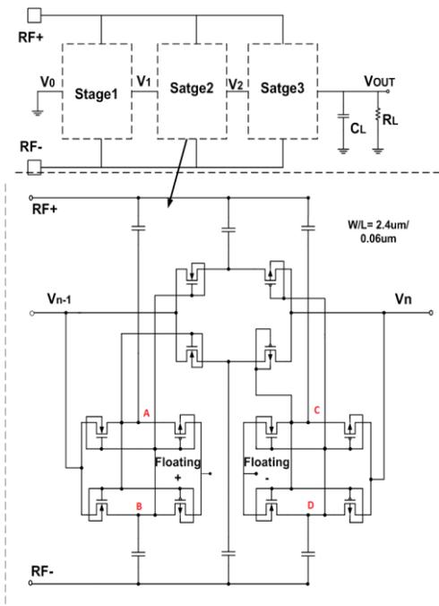
Fig. 2.4-1 Circuit of cross couple rectifier with DTMOS on 65nm SOTB technology.
