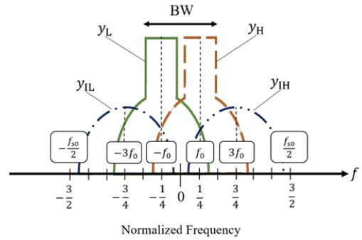
Fig. 2.2-8 Decomposed PA output spectra.
