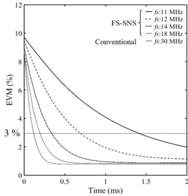
Fig. 2.2-11 Simulated EVM convergence v.s. sampling frequency
