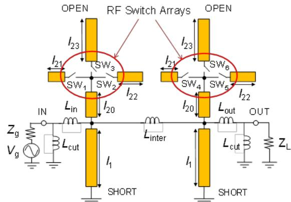
Fig. 2.2-3 Three-bit reconfigurable BPF with RF switch arrays.
