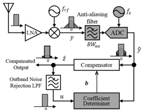
Fig.2.2-10 Proposed blind nonlinear compensation scheme with sub-Nyquist sampling technique.
