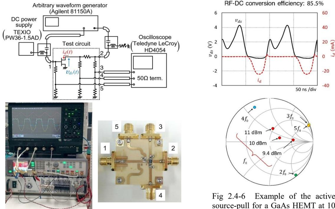
Fig. 2.4-5 MHz-band multi-harmonic active source-pull measurement system for estimating an intrinsic nonlinear resistance in a rectifying element
