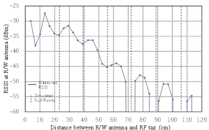
Fig.2.1-12 Measured height pattern of received power at R/W.
