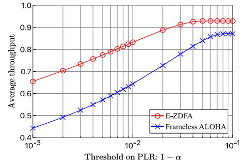
Fig. 2.3-8 Throughput of ZigZag decodable frameless ALOHA.
