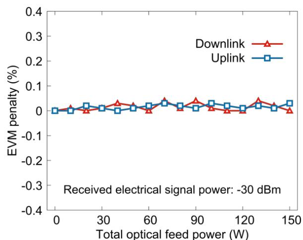
Fig. 2.3-11 EVM penalties to back-to-back signal of downlink/uplink transmitted signals into a 1-km DCF link while changing total optical feed power when received electrical power was set to  $-30$  dBm.
