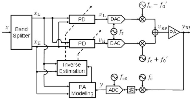
Fig.2.2-7 Block diagram of proposed DPD with band splitting method (Two-band splitting).
