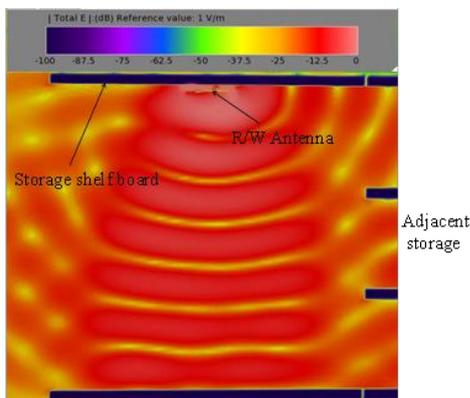
Fig.2.1-11 Electric field strength map in metal shelf.
