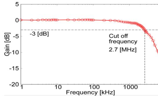
Fig. 2.4-7 : Frequency characteristics of PPC.
