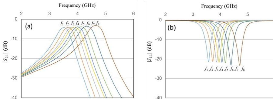
Fig. 2.2-6 Measured S parameters of prototype BPF, (a) S<sub>21</sub>, (b) S<sub>11</sub>.
