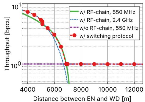
Figure 2.4-4: Throughputs of different communication schemes with and without RF-chain.
