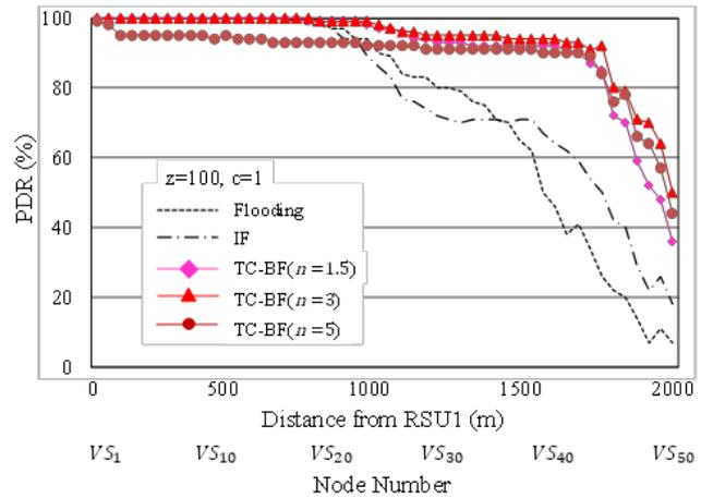
Fig. 2.1-5 Broadcast packet delivery rate (PDR) for 50 vehicle nodes on the straight road of 2 km.
