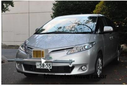
Fig. 2.1-9 Millimeter wave radar developed by Inaba Lab. of UEC
