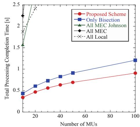
Fig.2.3-5 Total processing completion time as a function of number of MUs.
