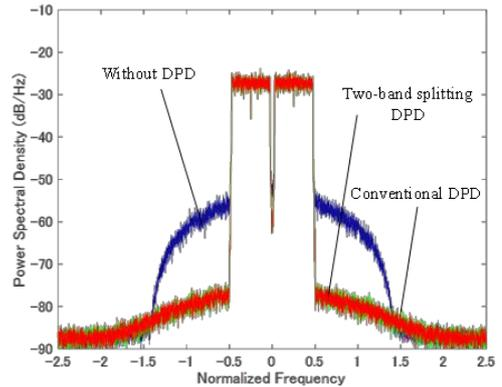
Fig. 2.2-9 PA output spectra with proposed DPD.
