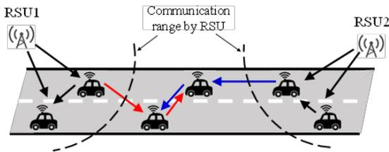
Fig. 2.1-4 Multi-hop road to vehicle broadcast communication.
