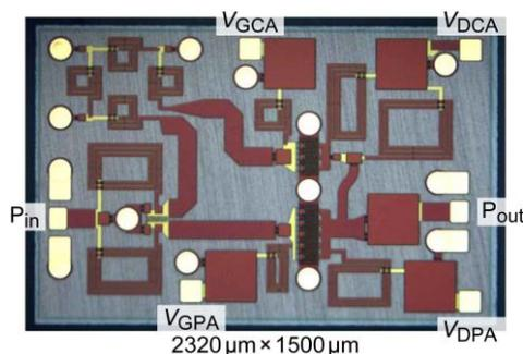
Fig. 2.2-1 4-GHz-band GaN HEMT MMIC asymmetric Doherty power amplifier
