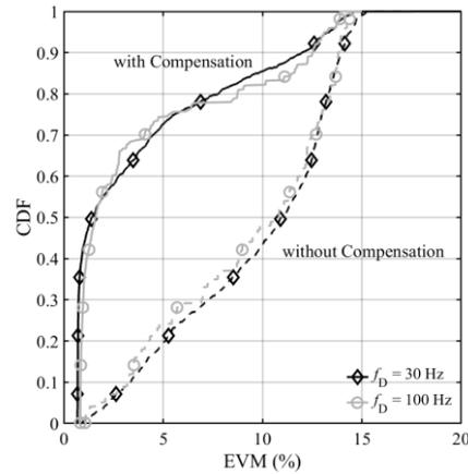
Fig. 2.2-12 CDF of EVM for Rayleigh faded channel ( $f_D = 30, 100$  Hz).
