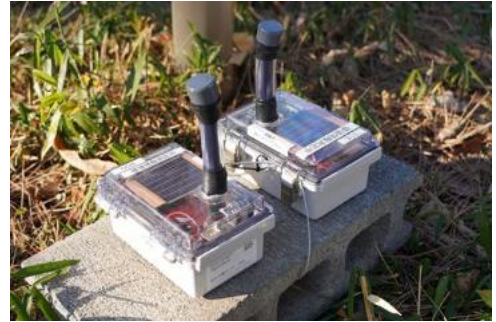
Fig. 2-4-3 wireless sensor node powered solely by solar EH and implementing the proposed ZEN-MAC protocol.
