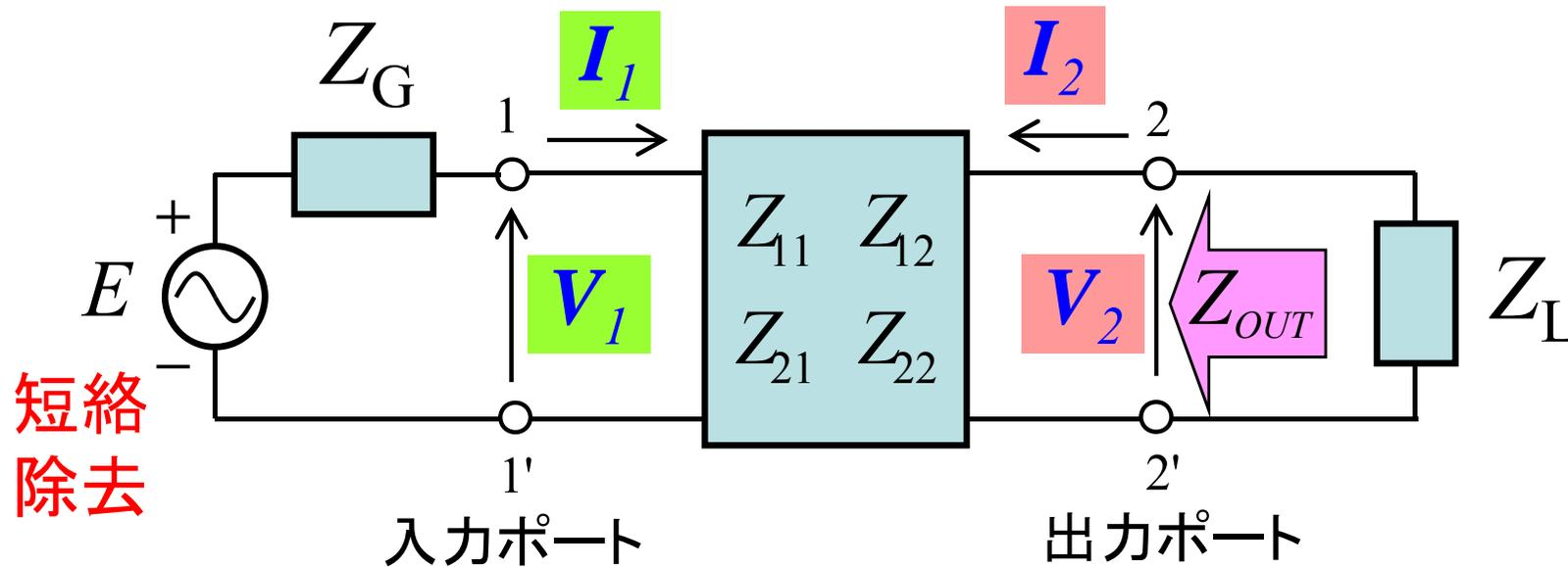
$$Z_{out} = \frac{1}{Y_{out}} = \frac{V_2}{I_2} \text{ より}$$
