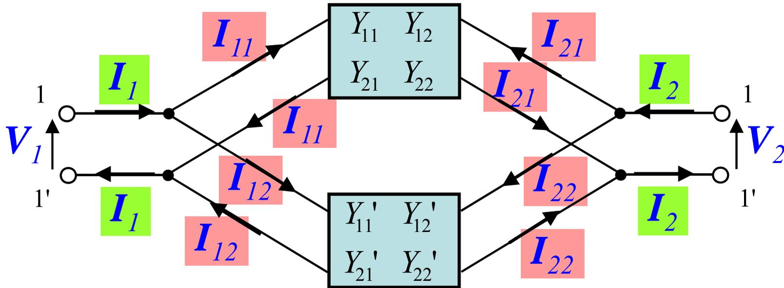
$$\begin{bmatrix} I_1 \\ I_2 \end{bmatrix} = \begin{bmatrix} I_{11} \\ I_{21} \end{bmatrix} + \begin{bmatrix} I_{12} \\ I_{22} \end{bmatrix} = \begin{bmatrix} Y_{11} + Y'_{11} & Y_{12} + Y'_{12} \\ Y_{21} + Y'_{21} & Y_{22} + Y'_{22} \end{bmatrix} \begin{bmatrix} V_1 \\ V_2 \end{bmatrix}$$
