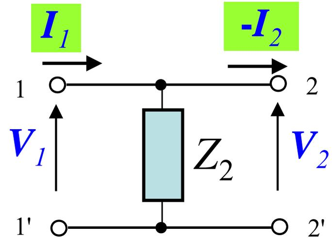
$$\therefore F = \begin{bmatrix} A & B \\ C & D \end{bmatrix} = \begin{bmatrix} 1 & 0 \\ \frac{1}{Z_2} & 1 \end{bmatrix}$$
