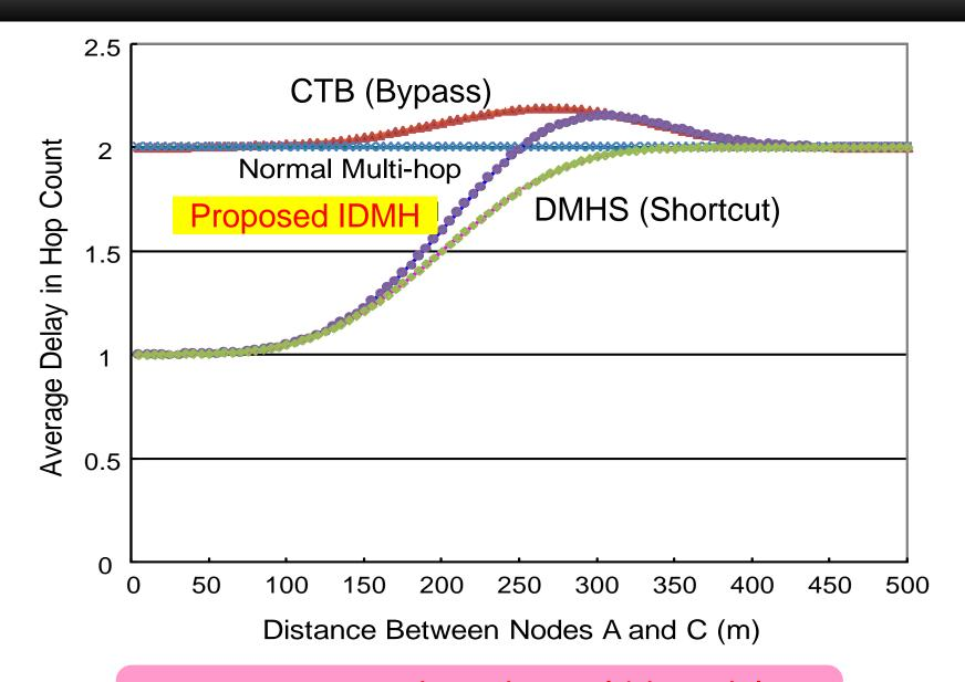
The IDMH can reduce the multi-hop delay when node distance is less than 250 m.
