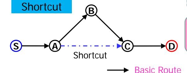
Multi hop Route should be dynamically changed according to the status of each Link
