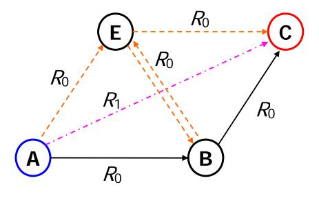
Nodes are located on a regular triangle lattice with the distance of  $R_0$  to the adjacent nodes.
