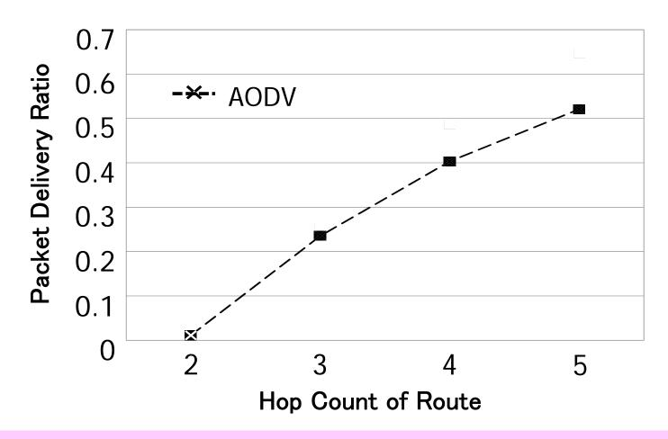
Routes with large hop count have better packet delivery ratio, although the ratio is still not good. To the contrary, multi-hop delay increases.
